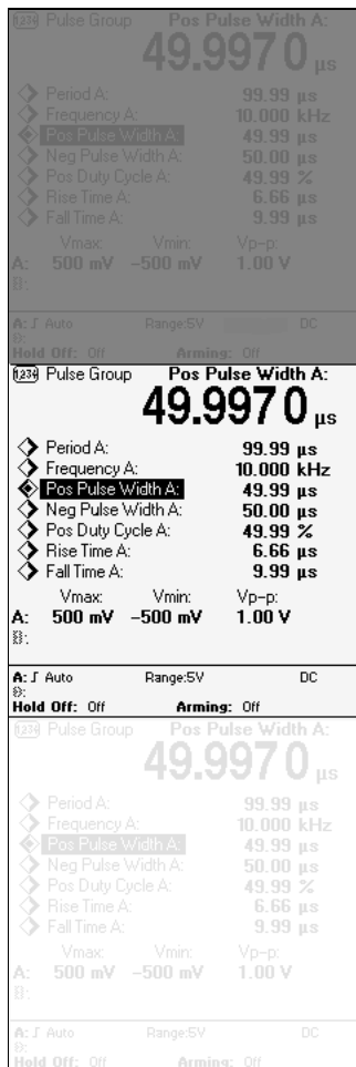
Figure 90 Display Contrast. The display contrast can be varied between 100% (top) and 0% (Bottom).
